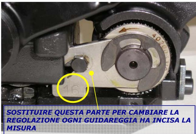
SOSTITUIRE QUESTA PARTE PER CAMBIARE LA REGOLAZIONE OGNI GUIDAREGGIA HA INCISA LA MISURA
